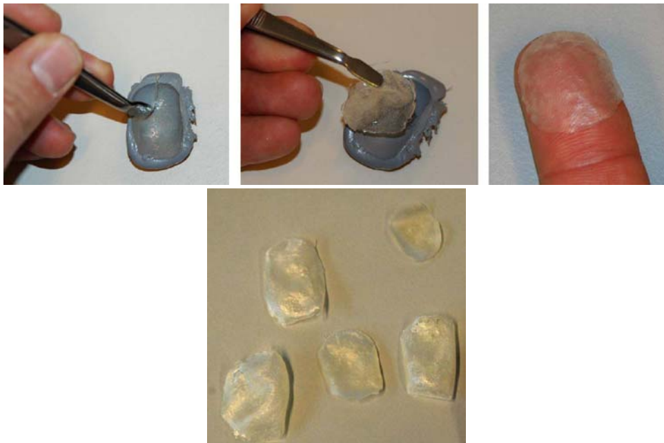
Figure 12. Silicon casts of fingerprints with silicon cast negative and acrylate paint as positive.
